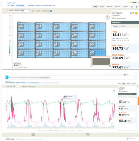
5. At least one month's panel production and optimizer voltage charts of the panel(s) being claimed and adjacent panels. These can be taken from the monitoring portal.
