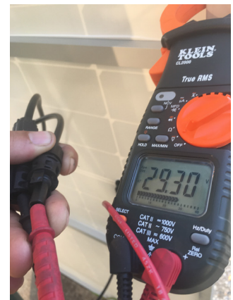
7. Module Voc multimeter measurement
